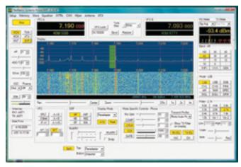
Figure 5 — You can split the *PowerSDR* screen to show any combination of the panadapter and waterfall displays.
